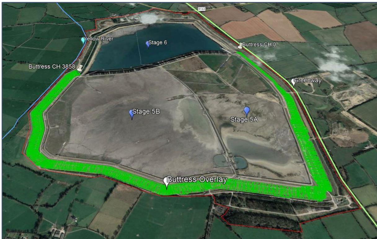
**Figure 2 Tailings Facility and Proposed Buttress Layout Plan**
